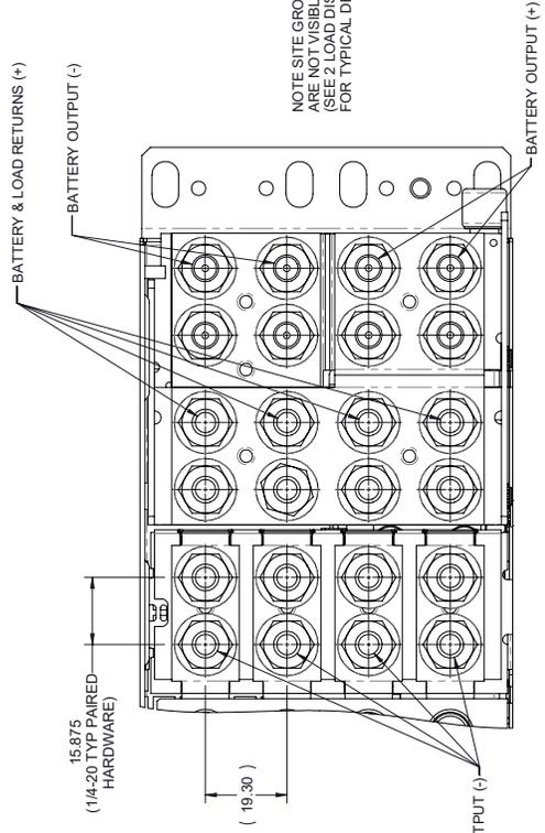
NOTE SITE GROUND TERMINALS ARE NOT VISIBLE IN THIS VIEW (SEE 2 LOAD DISTRIBUTION CONFIG. FOR TYPICAL DETAIL).
