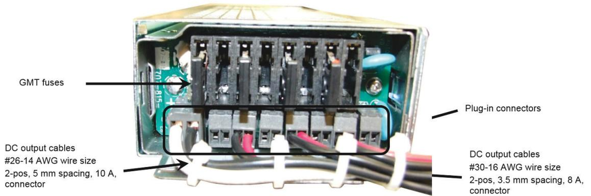
**NOTE:** Make sure the applicable fuse has been removed before unplugging the corresponding connector.
