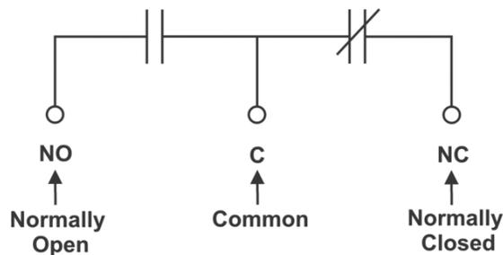
Relays can be programmed to energize or de-energize during an alarm condition (see controller software manual). When the CXCM1 reset button is pressed or power is lost, all relays de-energize.
