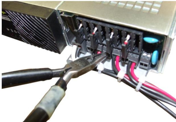
2. After the plug-in connector has been removed, attach the cables to the terminal block. Verify the polarity.
